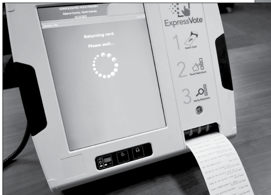
If a voter chooses to use the ExpressVote, their selections are printed on a paper ballot which they then insert into the ballot tabulator.
