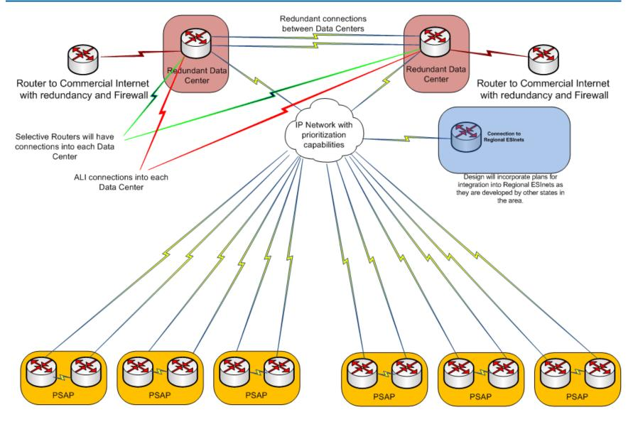
22 connected PSAP's with a connection to another PSAP for redundancy
